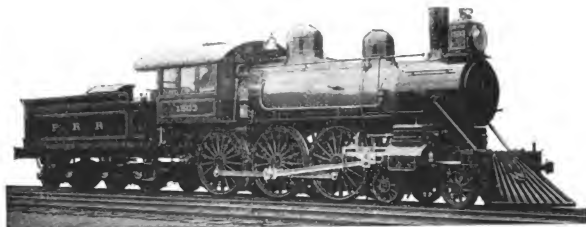
Fig. 62. Ten-Wheel (4-6-0) Two-Cylinder Schenectady Compound Locomotive. Built by the American Locomotive Co. for the Pennsylvania Railroad. Cylinders 20 in. and 30 in. x 24 in., Working Steam Pressure 180 lbs. per sq. in., Diameter of Drivers 74 in., Weight on Drivers 106,000 lbs., Total Weight 143,000 lbs.
